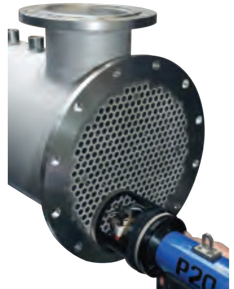
Automated tube end welding and 100% inspection
